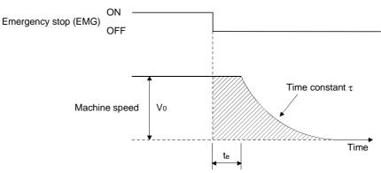
Fig. 11.2 Dynamic Brake Operation Diagram
